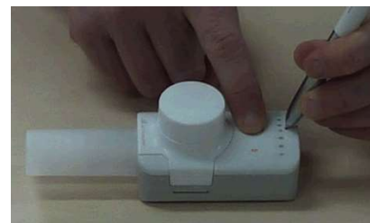
Figure 15: Press the “ON/OFF” key and the “inhalation time” key simultaneously using a pen to press the “inhalation time” key.
